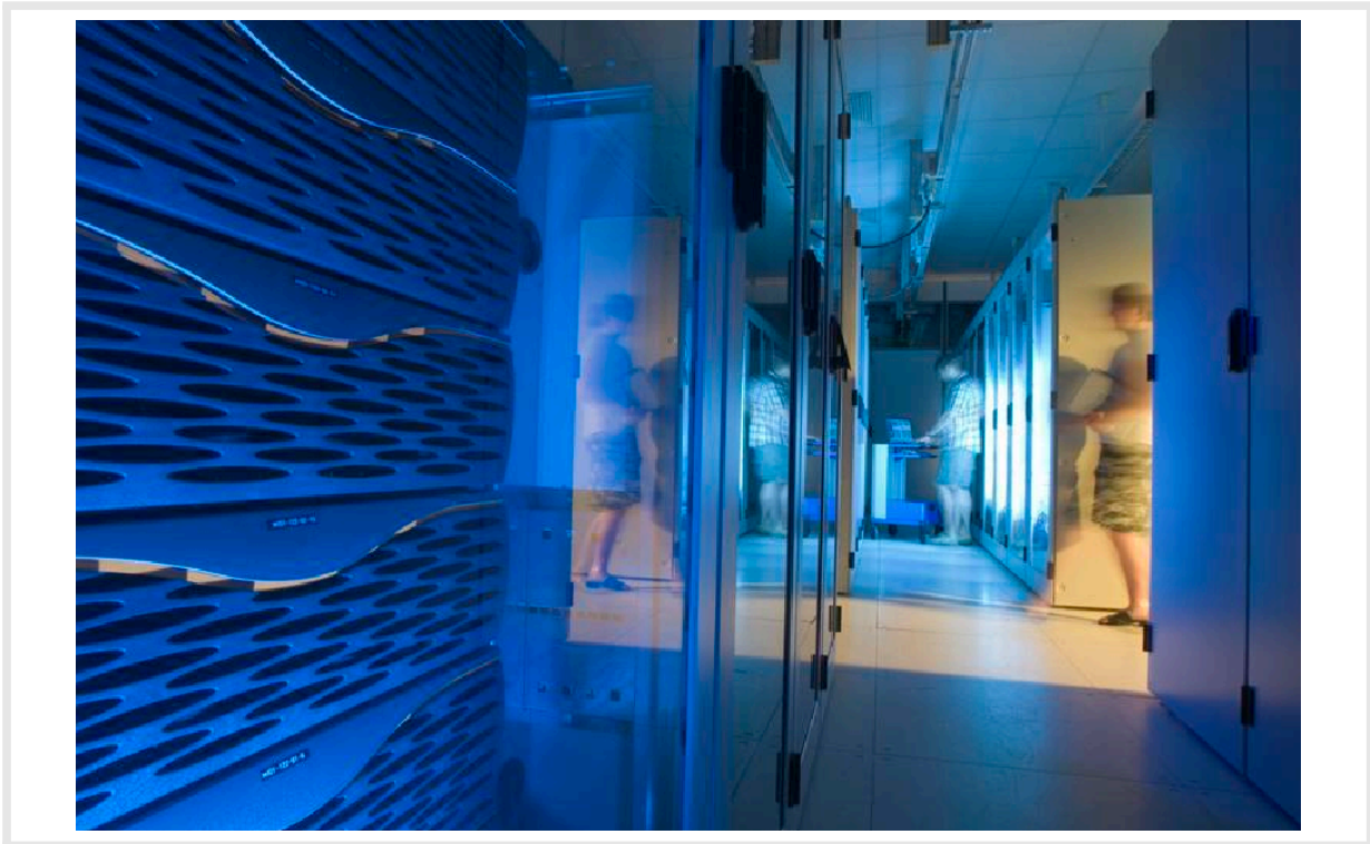
Figure 8.1.: The GridKa compute cluster is a Tier-1 centre in the academic EGI grid, located at Steinbuch Centre for Computing of Karlsruhe Institute of Technology. At the time of writing it comprised over 10000 CPU cores. (Picture used with permission from Steinbuch Centre for Computing)
